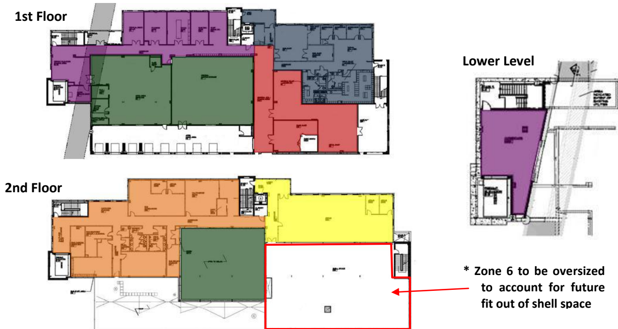
Figure 46: New Geothermal Zone Zones
