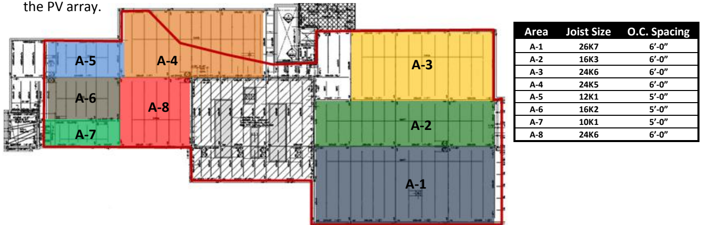
Figure 59: Main Roof Support Means & PV Array Boundary
